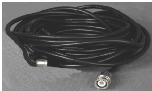
Fig 5-4 cable for all-direction antenna
